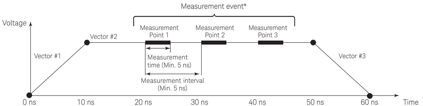
(\*) As well as the measurement event, the range change and trigger event can be specified in the vector.
