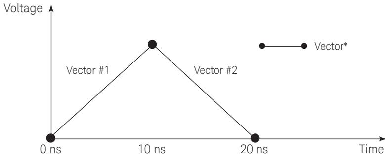
(\*) The waveform is created by specifying multiple vectors (time, voltage).
